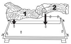
Figure 43 - Installing Logs No. 1 and No. 2
